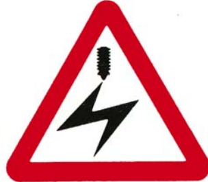
ELECTRIFIED OVERHEAD CABLE (safe height plate is to be added)
